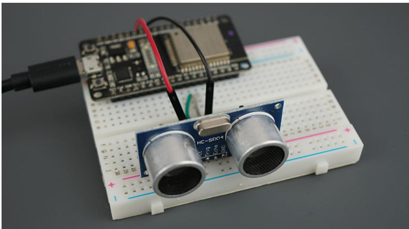
After uploading, open the Serial Monitor at a baud rate of 115200. Press the on-board RST button to restart the board and it will start printing the distance to the closest object on the Serial Monitor. Something as shown in the picture below.
