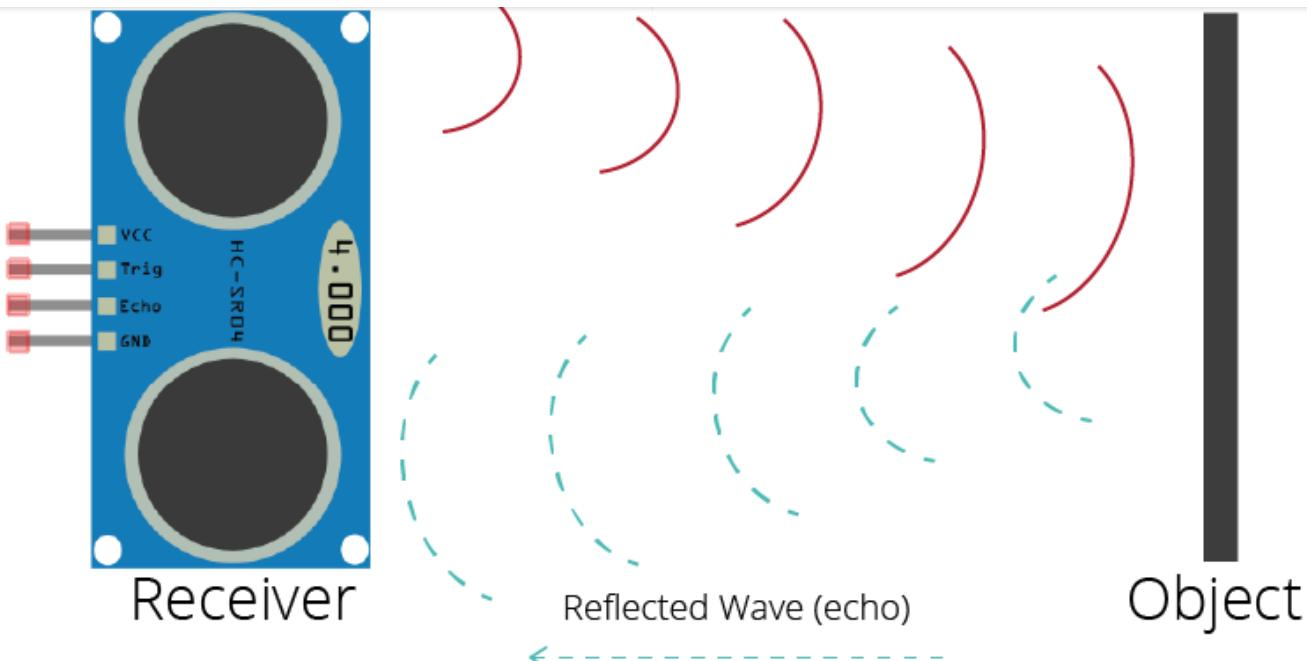
Taking into account the sound's velocity in the air and the travel time (time passed since the transmission and reception of the signal) we can calculate the distance to an object. Here's the formula:
