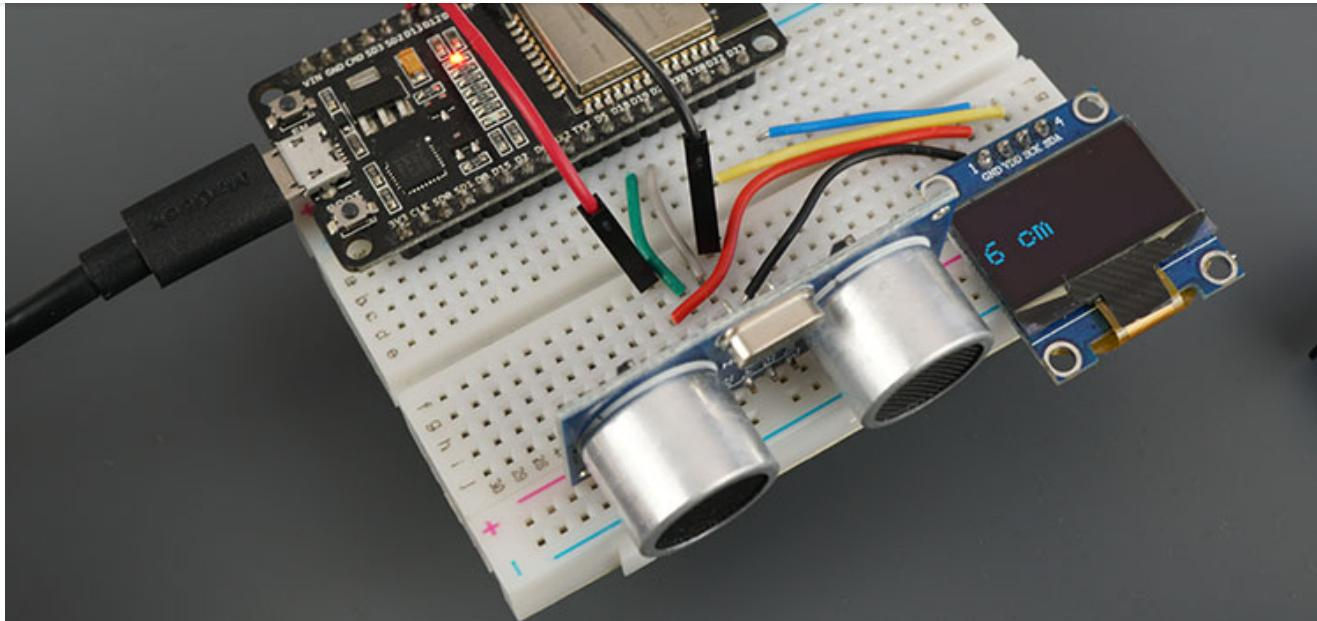
In this section, we'll show you a simple example with the ESP32 that displays the distance on an I2C OLED display.
